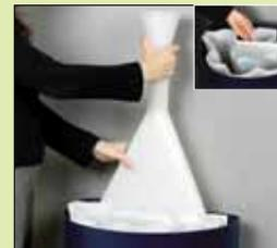
Remove the reservoir unit located at the back of the cup bank for emptying. Re-position the reservoir unit against the back wall of the cup bank.
